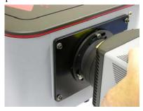
**2.** Finger tighten three hex head screws into the mounting plate. Leave about <sup>1</sup>/<sub>4</sub>" thread exposed.
